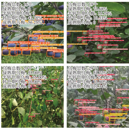
图 7 改进 YOLOv7—1 网络模型的乌梅不同成熟度检测效果 Fig. 7 Detection effect of the improved YOLOv7—1 network model on different maturity of black plum
